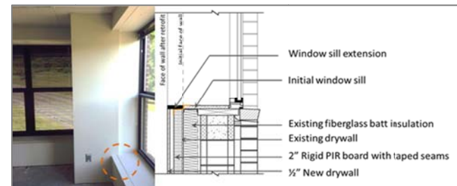
Figure 7: Extended window sill over additional retrofit components
