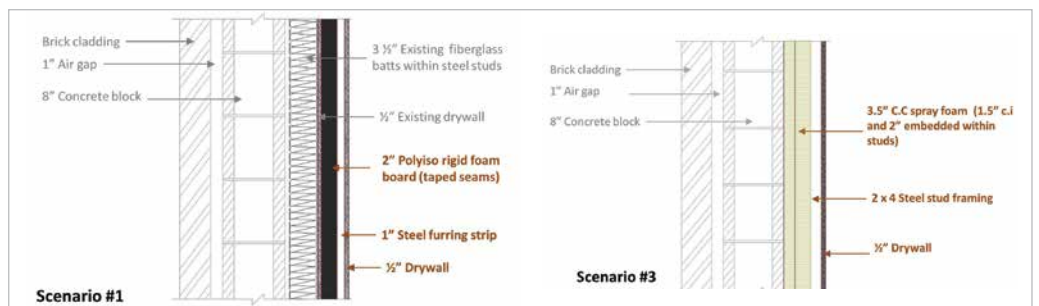
The two retrofit scenarios, down-selected for field demonstration through this project, were installed in two of the eight zones in the FRP.
