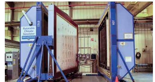
A wall air and moisture penetration test chamber and a rotatable guarded hot box were used in the laboratory to test full-scale assemblies.
