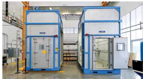
A wall air and moisture penetration test chamber and a rotatable guarded hot box were used in the laboratory to test full-scale assemblies.
